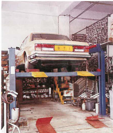
Fitting a new full set of the exhaust system to a Rolls Royce at Hing Yu's service centre.
